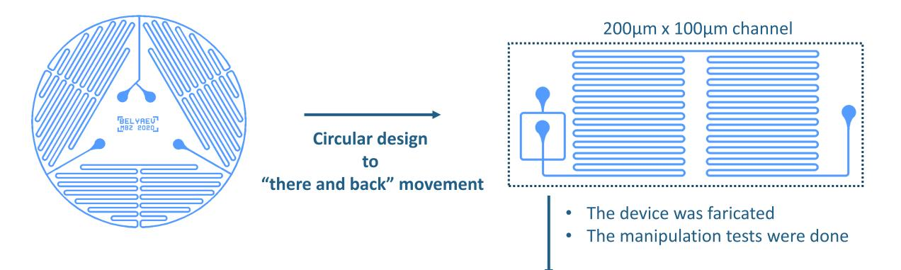
An array of ~100 droplets is generated and guided over the sensor area in "there and back" manner. The time duration of **one cycle is about 5 minutes**. **Maximum** achieved **3 hours and 30 minutes total incubation** of ones generated droplets.
