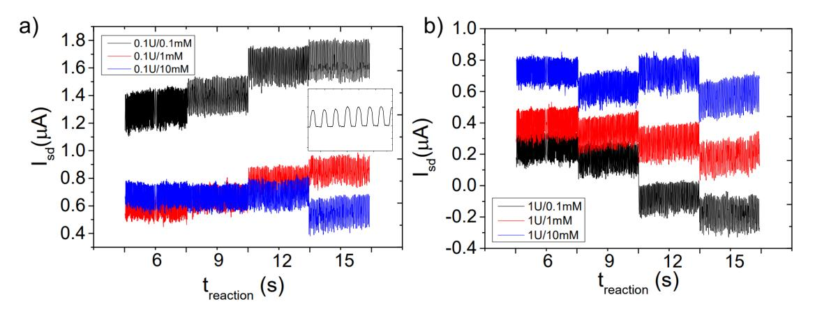
Data obtained from the assay with the subtracted effect of streaming potential. (a) Reaction with increasing substrate concentration and constant enzyme concentration at (a) 0.1 U and (b) 1 U.
