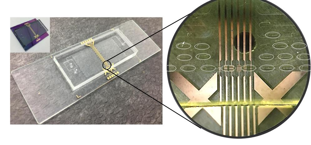
Permanently sealed device: 200  $\mu$ m X 100  $\mu$ m channel, 6 electrode sensors on board with 6, 12 and 18 interdigitated micro-wire pairs (each duplicated).
